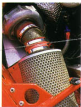
Turbo breathes through ventilated dustbin. Not the same dustbin that the Xantia trim went into
